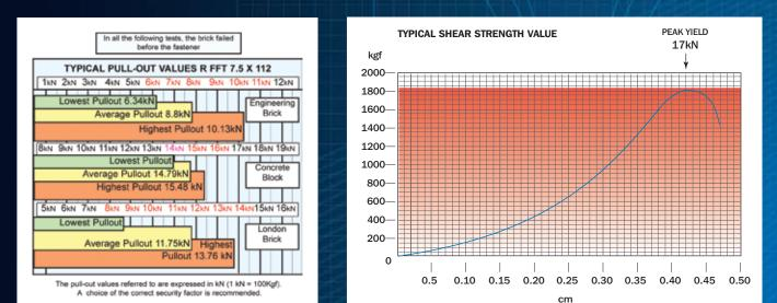
\* Average pull out figures are typical values and ultimate pull out will be dependent on the condition of the material. It is recommended that any user establish the nature and condition of any substrate prior to useage.
